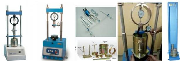
Figure 4. From left to right: CBR Test Machines with capacity (50 kN) fit for EN 13286-47, BS 1377:4, ASTM D1883, AASHTO T193, NF P94-078, UNI CNR 10009 standards; parts of moulds and gauges, ongoing tests, and compactor machine.
